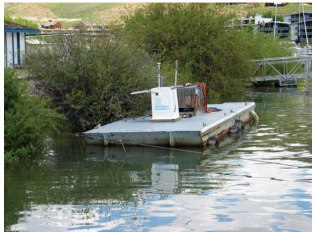
Figure 19 - Sanitary Pump Out Barge (2)
