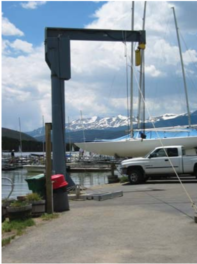
Figure 16 - Boat Lift Crane (5,000 lb. capacity)
